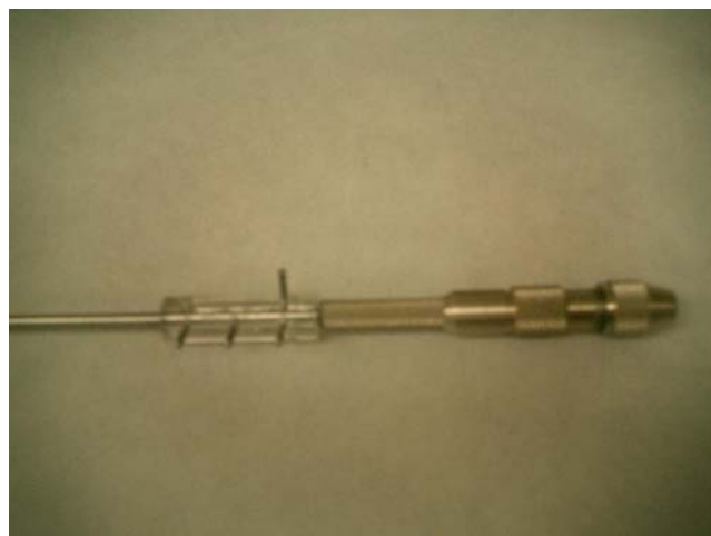
Figure 3.21: The fiber clamp of the fiber insertion system consists of an aluminum fiber clamp tube, in which the optical fiber is inserted, a plexiglas fiber clamp handle, an aluminum pin vise, and four stainless steel dowel pins. The two pins nearest the distal end are locking pins. The other two pins are rotating pins. As with the trocar, these rotating pins are used to both lock / unlock the fiber clamp and retract / insert the clamp. The inner diameter of the tube was chosen to allow insertion of a 2 cm diameter diffusing tip optical fiber. The fiber clamp tube is inserted into the cannula once the trocar is removed. The optical fiber is inserted through the pin vise, which clamps the fiber after insertion.
